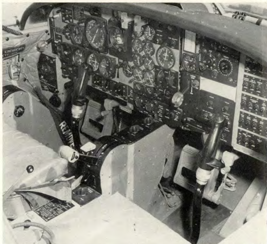
The T-37 has dual flight and power controls and the student's side has the standard instruments.
