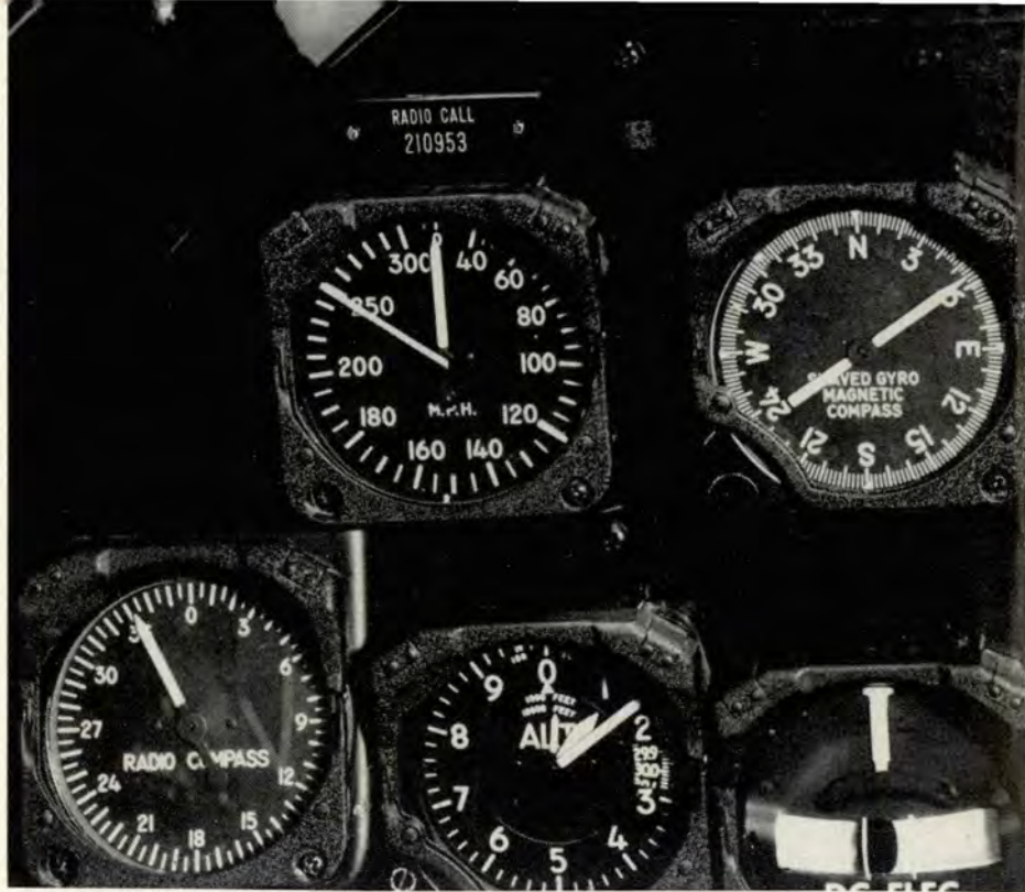
On the ADF, turn right and needle moves left. Remote indicating compass works the other way. Use these instruments on beacon letdown and you'll know what it's like to be mentally crosseyed.
