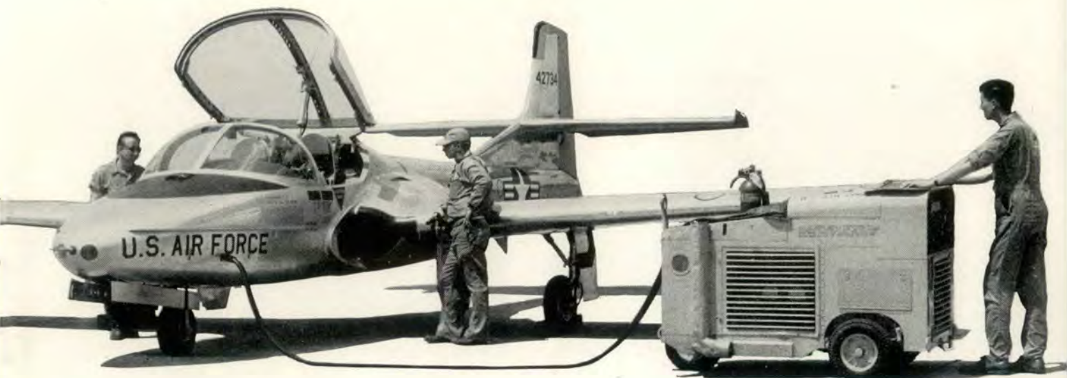
Note starting unit receptacle. The T-37 measures nine feet to top of stabilizer.
