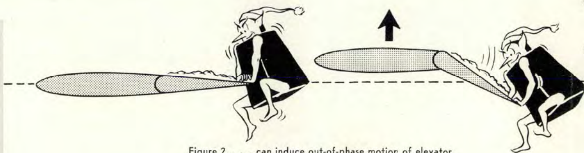
Figure 2. . . . can induce out-of-phase motion of elevator.
