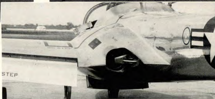
Close-ups of the tailpipe area show how the thrust attenuators appear; extended and retracted.
