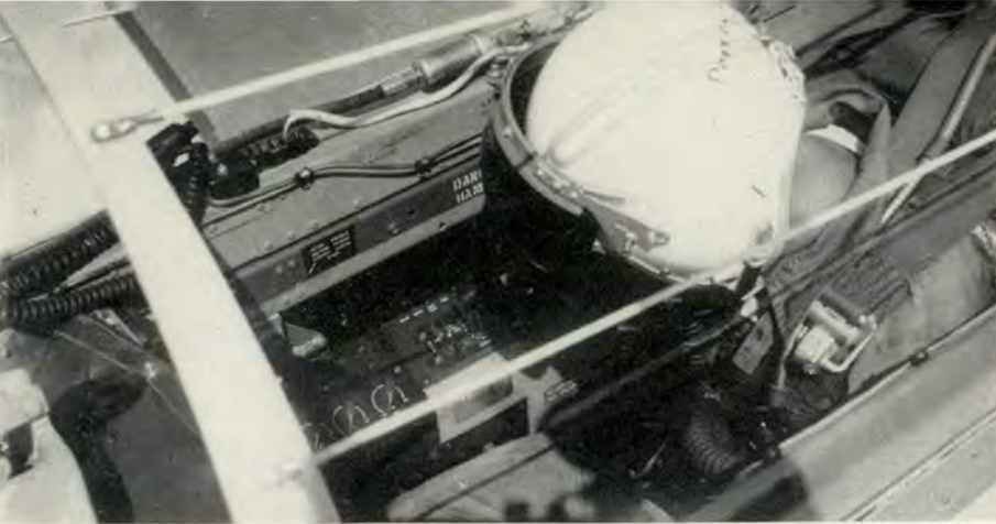
When IFR, duck your head down and to the side to select channel. A perfect set-up for vertigo.
