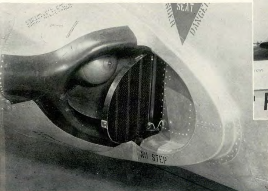
Screens cover the intakes when the wheels are down. They retract automatically with "gear up."
