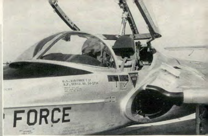
A stall spoiler generates natural stall warning.
